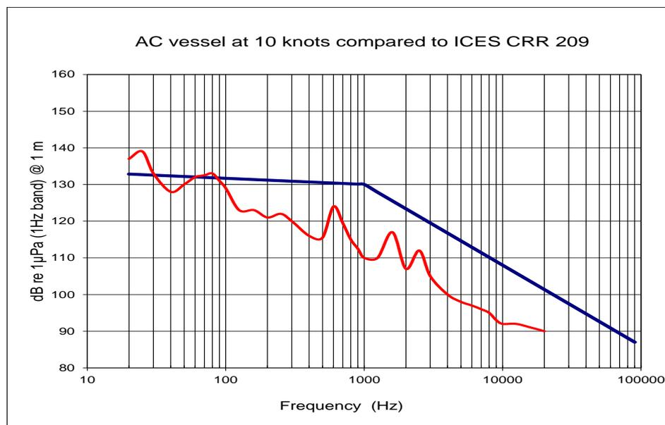
**Figure 10 – Spectrum level of a RV with AC motors at 10 knots**
