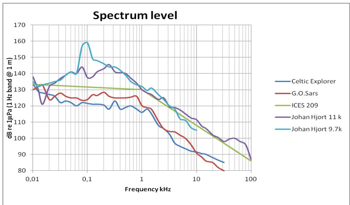
The measurements are done when the vessels pass over a deployed hydrophone at a distance of about 100 m. The levels are averaged in 1/3 octave band, "normalized" to 1 Hz band. "Johan Hjort" has a CPP which is optimized at a speed of 11 knots. The level below 1 kHz is dominated by noise from the diesel engine.
