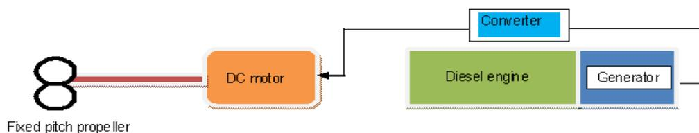
**Figure 5 – Diesel electric (DC) propulsion system**
