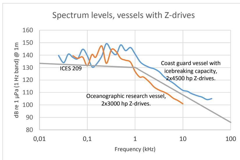
Figure 11 – Examples of vessels with Z-drive propulsion
