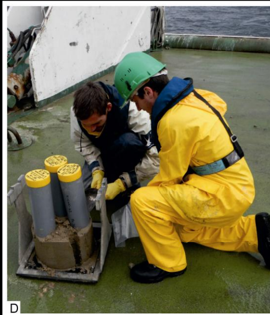
Box-core described and subsampled
