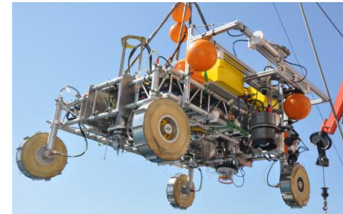
Crawler-System: Micro-Profiler (autonomous or real-time mode)
