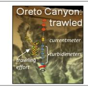
Schematic not scaled graphs of the deployed ISLAND mooring. Yellow dots indicate the highest trawling effort along the Oreto Canyon (Palermo).
