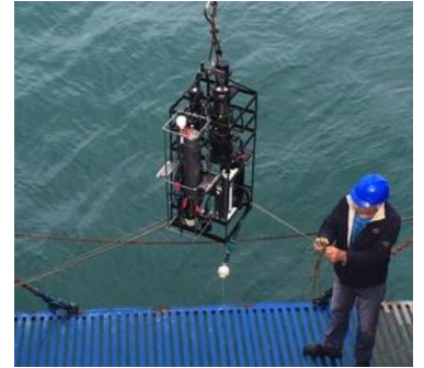
Deploying Optics Cage to measure Inherent Optical Properties (Absorption, Attenuation and Backscattering)
