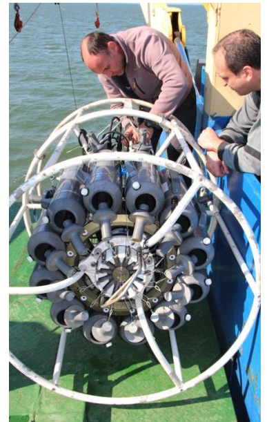
CTD Rosette System, with twelve five sample bottles
