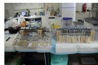
Pore water sampling from sediment cores taken with the box corer at active seep sites and deep-water coral sites (copyright A. Foubert)
