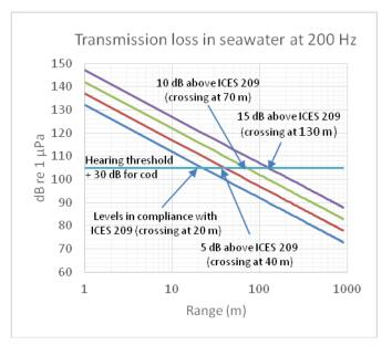
Figure 7 - Transmission loss in seawater with spherical spreading
