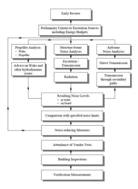
Figure 9 – Noise control plan (courtesy of DnV GL)
