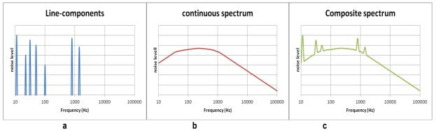
Figure 6 – a) Line component spectrum. The line frequencies are typically: blade frequency and harmonics, cylinder firing frequency, alternating current frequency, noise from reduction gear and slot frequency (windings in rotors passing gaps in the magnetic fields).
