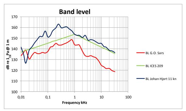
Figure 3 – URN signatures of "Johan Hjort " (11 knots) and "G.O. Sars" together with the ICES 209 line presented as band levels.
