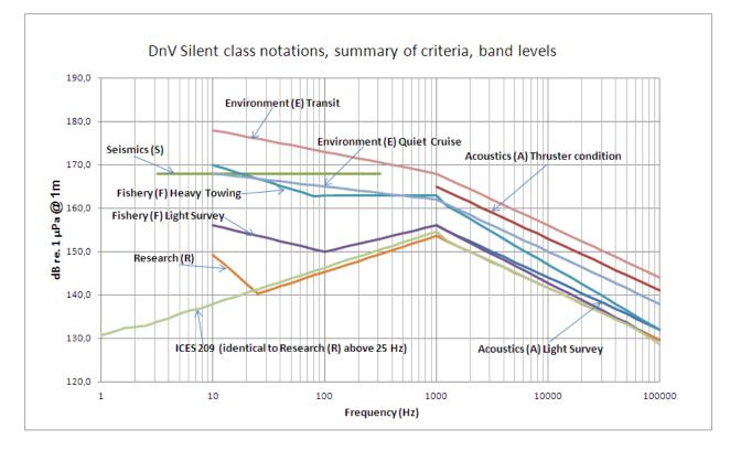
In Figure 8, a summary of the levels specified in the DnV GL Silent class notation is shown.
