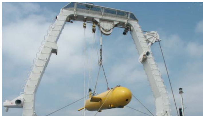
Fig. 4.2.3.2.f - Frame winch with fairleader blocks. (Travelling block) (Photo Ifremer)
