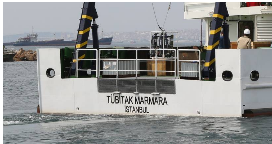
Fig.5.1.3.a - Step Deck & Stern Platform on R/V TUBITAK MARMARA. (Photo TUBITAK)
