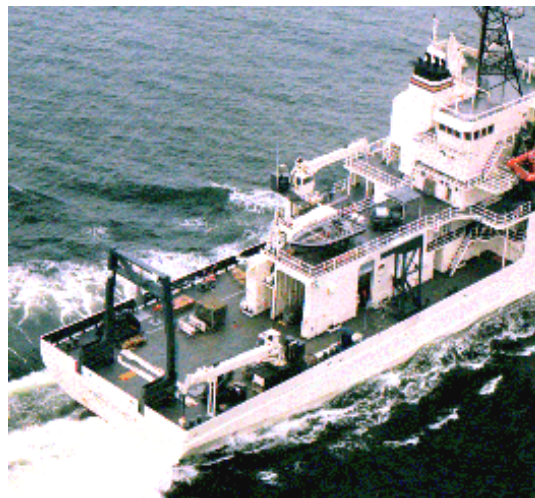
Fig.4.2.2.d - View of the work deck of R/V Thomas G. Thompson with centre hangar. (Photo: U. of Washington)
