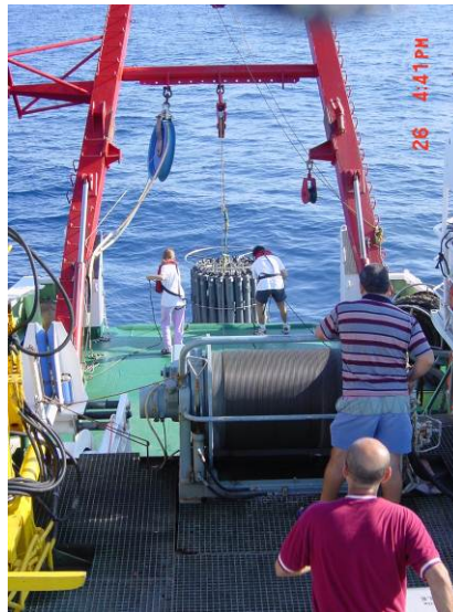
Fig 3.1.6.a - Astern deployment of CTD-Rosette. RV Garcia del Cid. CSIC. (Photo UTM)
