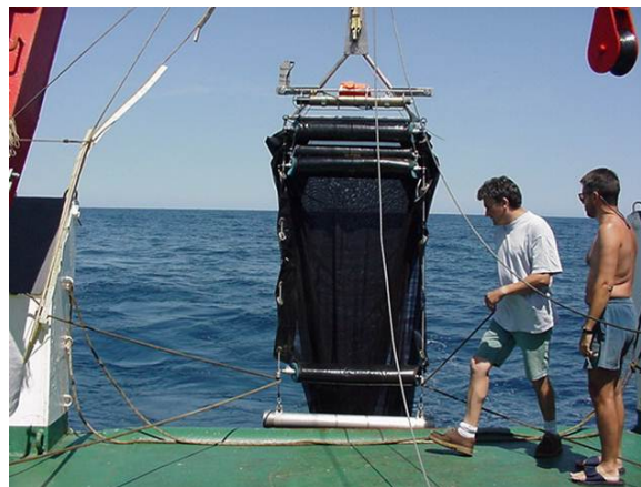
Fig.3.2.4.b - 1 m 2 RMT with mechanical release, controlled with electromechanical cable or acoustically. (Photo UTM)
