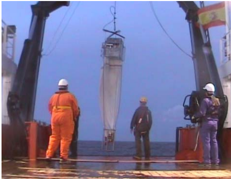
Fig.3.3.3.a - MultiNet deployment astern. (Photo UTM)
