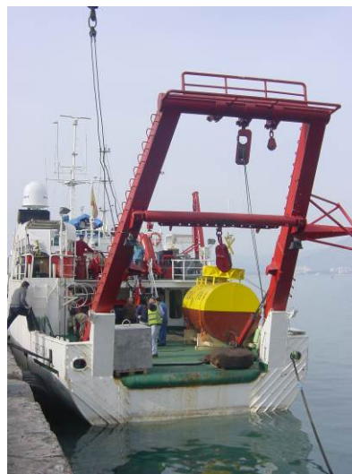
Fig. 4.1.4.a - Buoy ready for deployment on R/V García del Cid. (Photo UTM)
