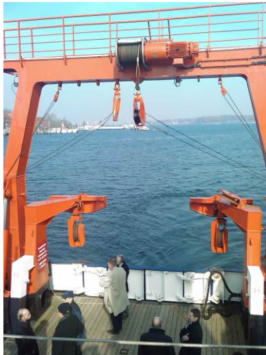
Fig. 4.2.3.2.d - Alkor (IFM-GEOMAR) aft frame. (Photo UTM)
