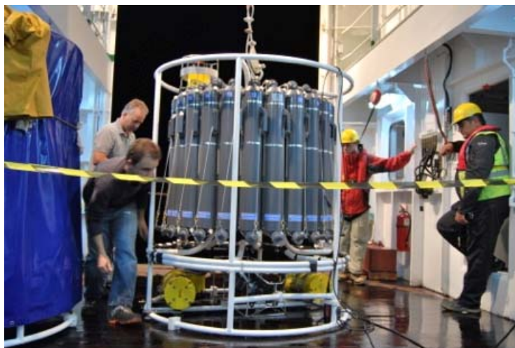
Fig. 3.1.1.a - CTD-Rosette on board RV Sarmiento de Gamboa (Photo: UTM)
