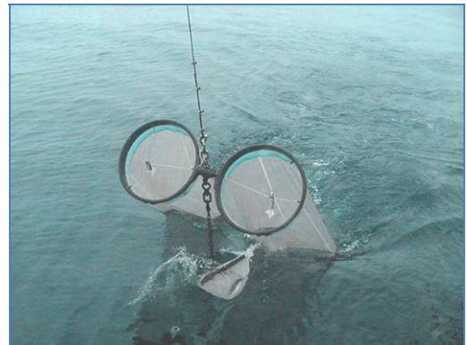
Fig. 3.2.1.b Flowmeters in the mouth of the net (Photo I. Palomera)
