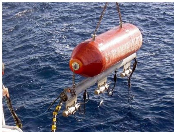
Fig. 3.11.2.b - Example of airgun array for high resolution seismic work. (Photo Ifremer)
