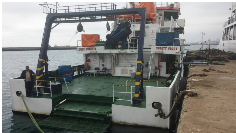
Fig. 5.1.3.d - Step Deck & Stern Platform on R/V TUBITAK MARMARA. (Photo TUBITAK)
