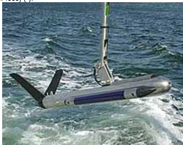
Fig. 3.10.1.a - The Klein tow fish, which performs Side-Scan SONAR, being pulled out after a survey. (©Klein Sonar Associates)
