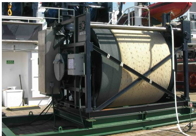
Fig.4.2.4.1.c - Moveable undulating CTD winch on beams on deck (Photo UTM)
