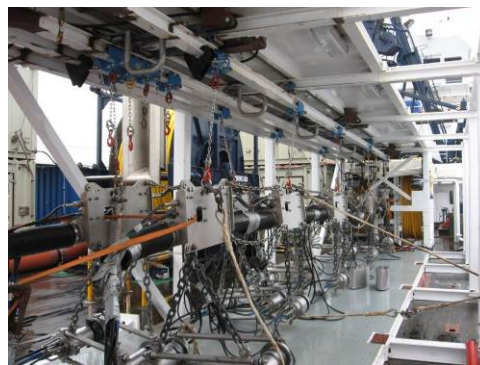
Fig. 4.2.1.c. - Airgun array structure. (Photo UTM)
