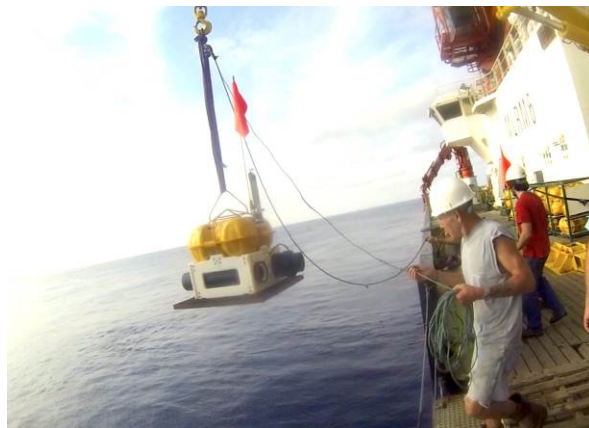
Fig.3.15.1.a - Launching an OBS from the deck of RRS James Cook. (Photo UTM)
