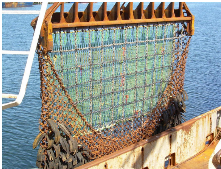
Fig. 3.9.2.a - Example of a fishing dredge (Photo NOAA)
