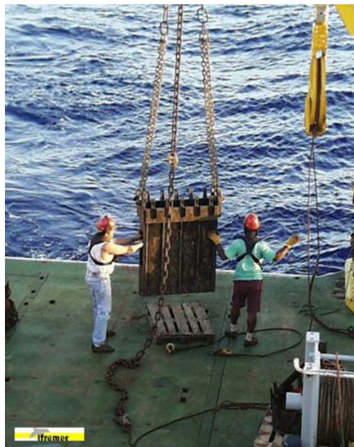
Fig. 3.9.1.a - Examples of rectangular dredge (Photo Ifremer)
