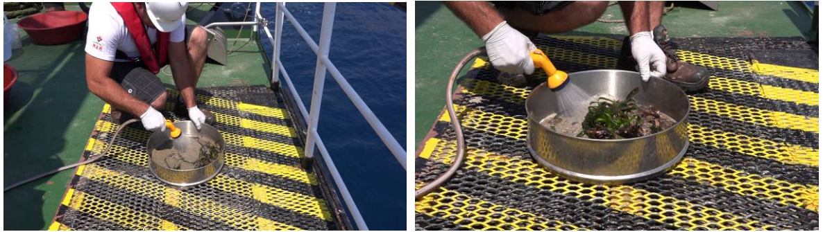
Fig.5.1.3.c - Sediment Sample Water Drainage Stern Platform on R/V TUBITAK MARMARA. (Photo TUBITAK)
