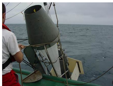
Fig. 3.3.1.b Deploying the LHPR. (Photo UTM)
