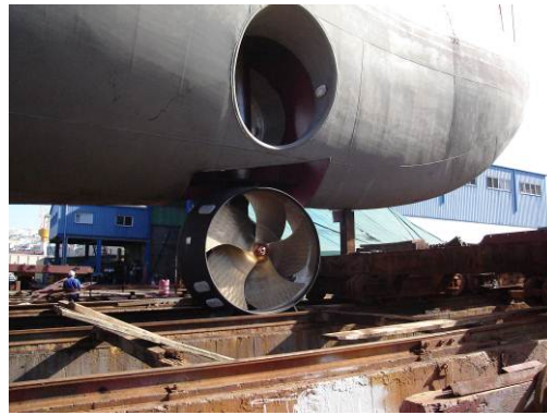
Fig. 4.1.1.a - Azimuthal bow thruster. (Photo UTM)
