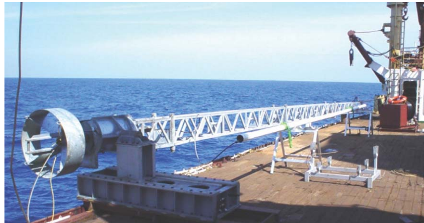
Fig. 3.8.7.a- A corer on Pelagia (Photo NIOZ)
