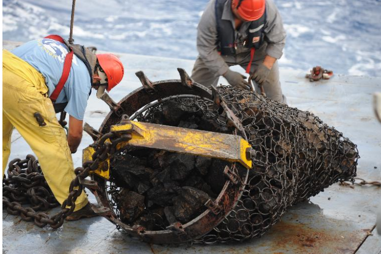
Fig. 3.9.1.b - Examples of cylinder dredges (Photo Ifremer)
