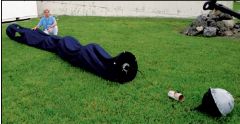
Figure 3.14.1.a - Each SVP drifter weighs 20 kg (44 lbs). Before deployment, the drogue and tether are bound with paper tape, which dissolves in the water, and the tether is sometimes wrapped around a water-soluble cardboard tube to protect it from kinking.
