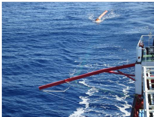
Fig.4.2.1.b - Boom for moving an airgun array aside. (Photo UTM)
