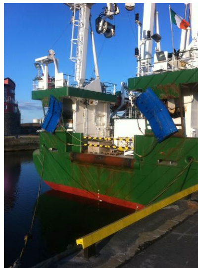
Fig.4.2.2.b - Aft A-frame installed over spare decks on R/V Celtic Explorer. Note the doors stowed on these structures. (Photo UTM)
