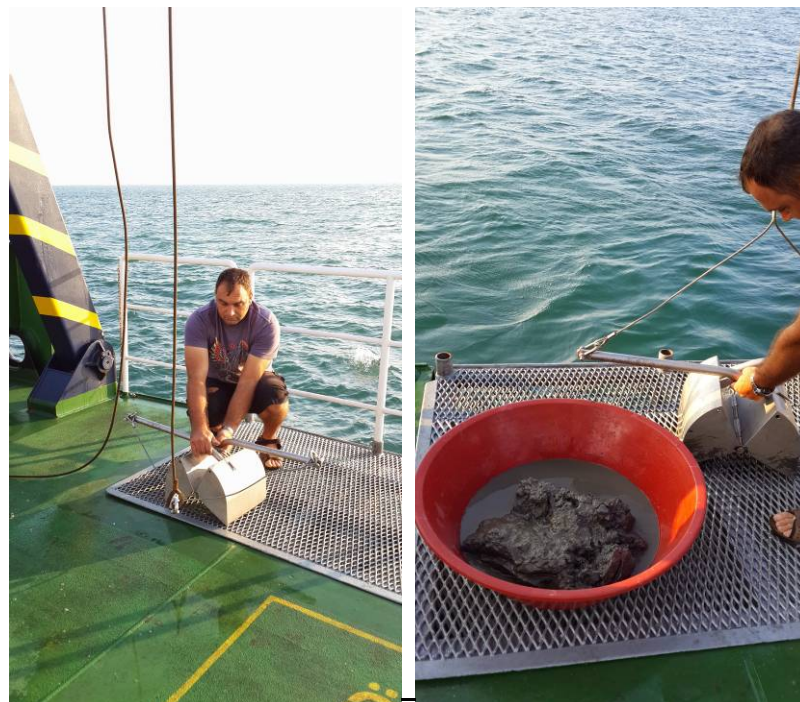
Fig.5.1.3.b - Sediment Sample Discharge and Drainage Stern Platform on R/V TUBITAK MARMARA. (Photo TUBITAK)
