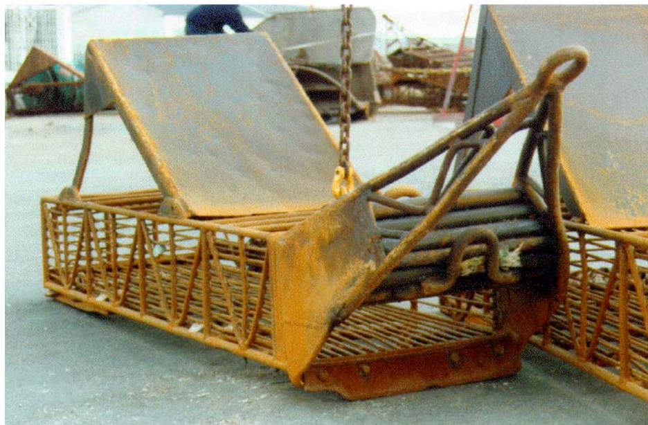
Fig. 3.9.2.b - Example of an Agassiz dredge (Photo Ifremer)
