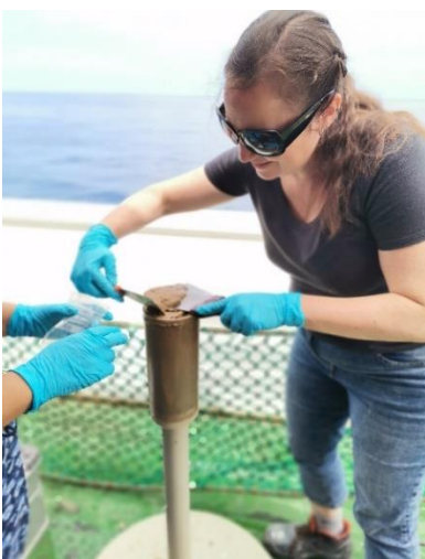
Fig. 4.14 Core liner (recovered from the box-core) being subsampled on board for DNA and RB analysis.
