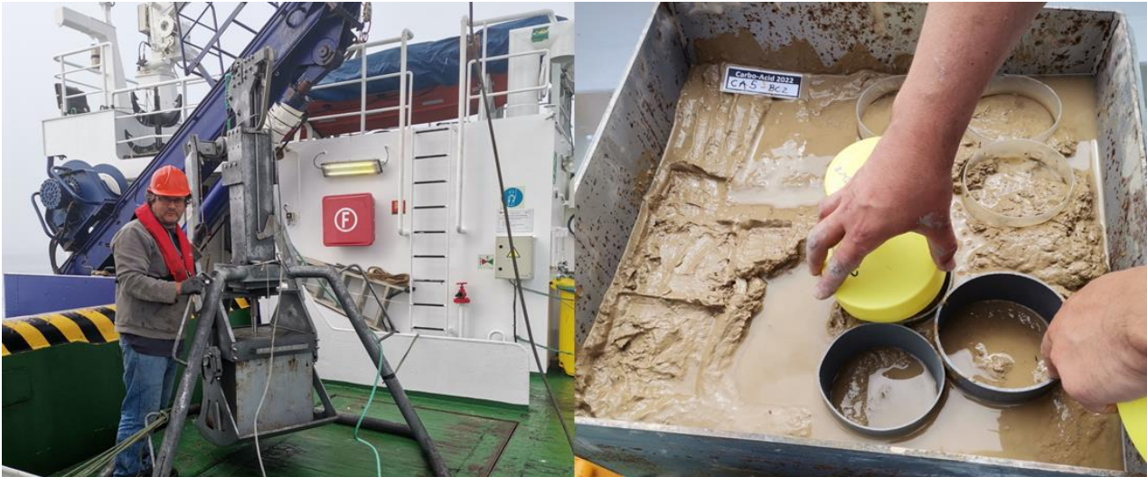
Fig. 4.13 Box-corer (left) and sediment box with push liners being recollected (right).
