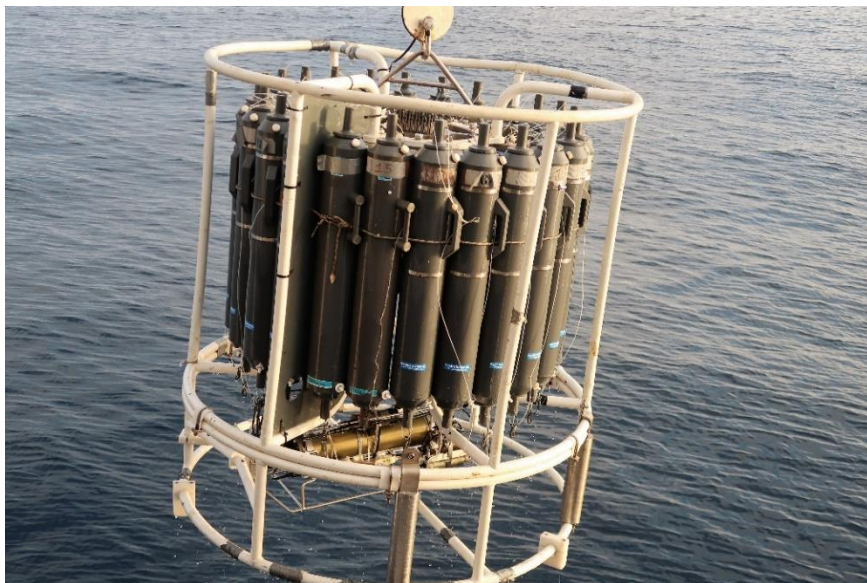
Fig. 4.6 Seabird-CTD-system 2x SBE 911 Plus mounted on a rosette used in the CARBO-ACID cruise.
