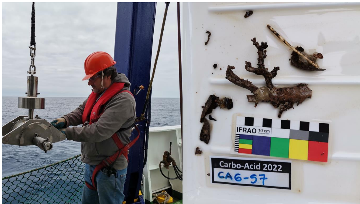
Fig. 4.12 Shipek grab being operated during the cruise (left) and recovered sample at station CA6.
