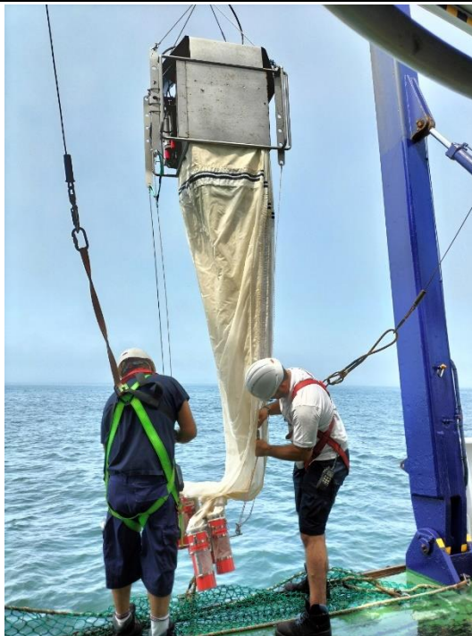
Fig. 4.10 During the CARBO-ACID cruise, samples of planktonic organisms were collected with a HYDRO-BIOS multi plankton sampler MultiNet, type Midi with five zooplankton nets, using vertical tows.
