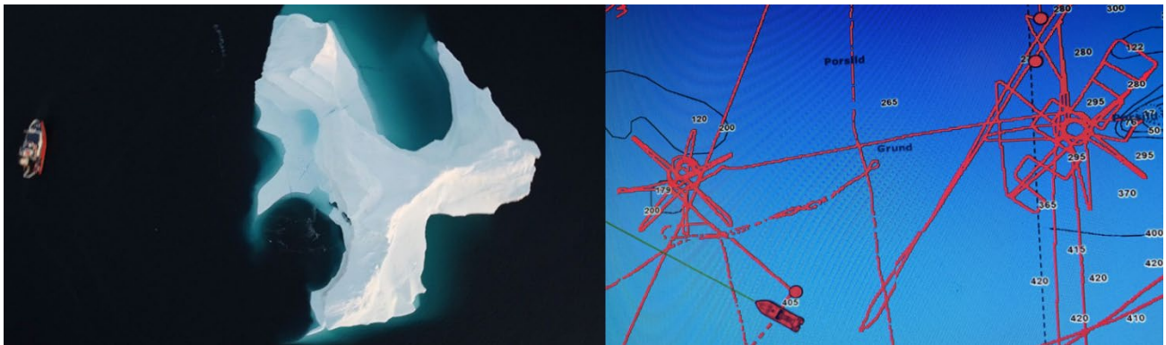
Fig. 3. Iceberg operations at “Muskox” and “Narwhale”. Drone footage was used to constrain the dimensions of the icebergs (left) whilst radar was used to conduct a regular survey of the iceberg periphery (right).
