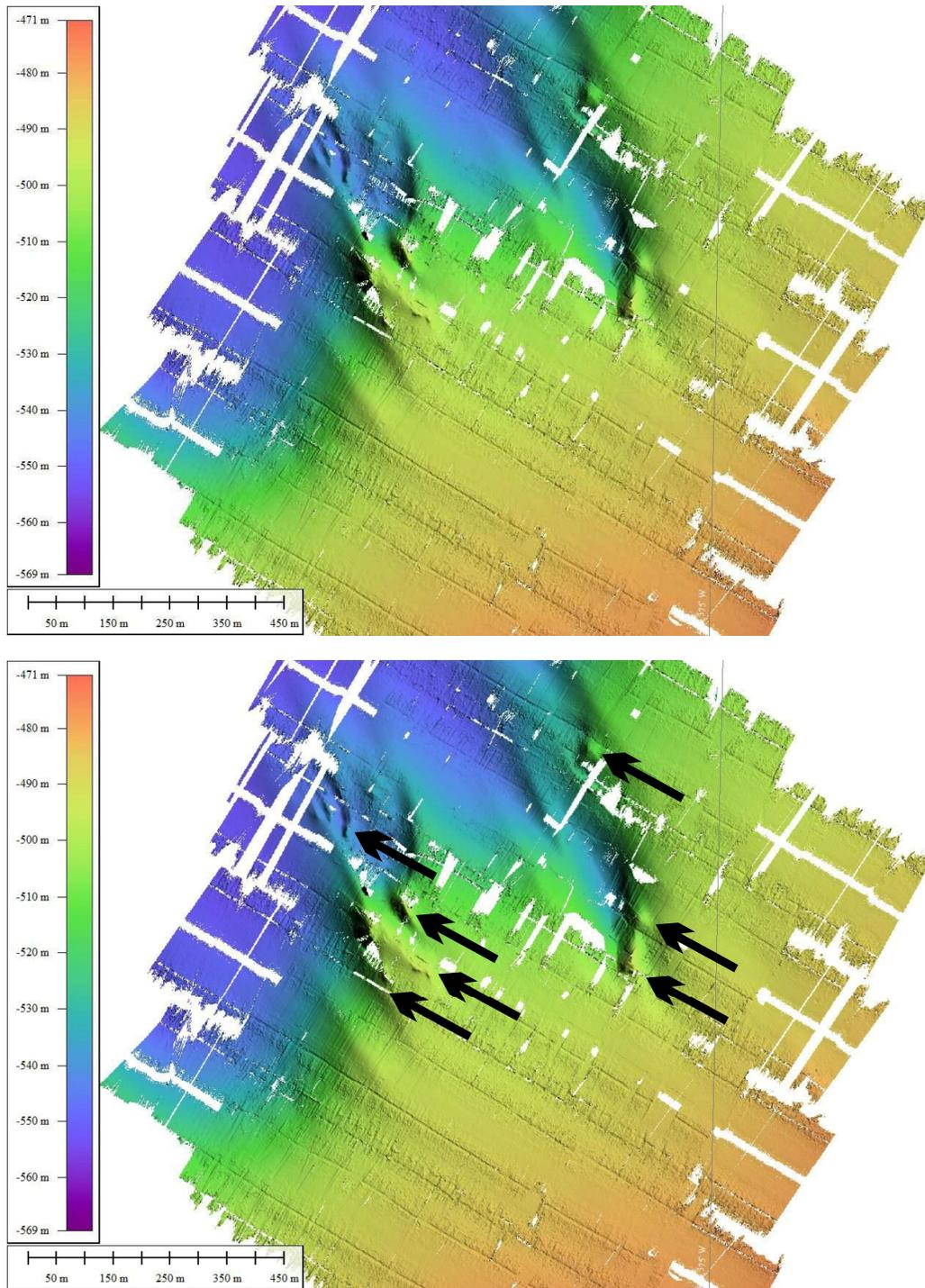
**Fig. 19** A) Capture of the interferometric bathymetry map obtained by the VLIZ team in target area 2 (AUV dives 2.1 and 2.2), based on the side scan sonar data. B) The coral mounds detected in the area are highlighted for clarity.
