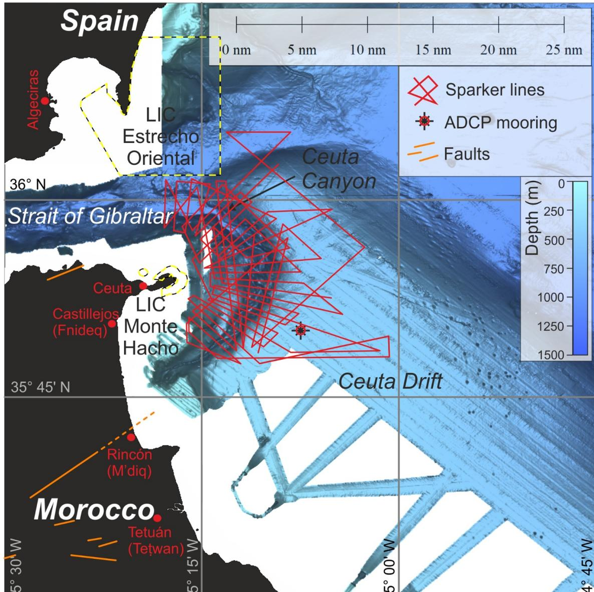
**Fig. 1** Working area and Sparker track chart of R/V BÉLGICA Cruise 2022/11. Bathymetry from the CONTOURIBER Project (Published in *Somoza et al., 2012*).
