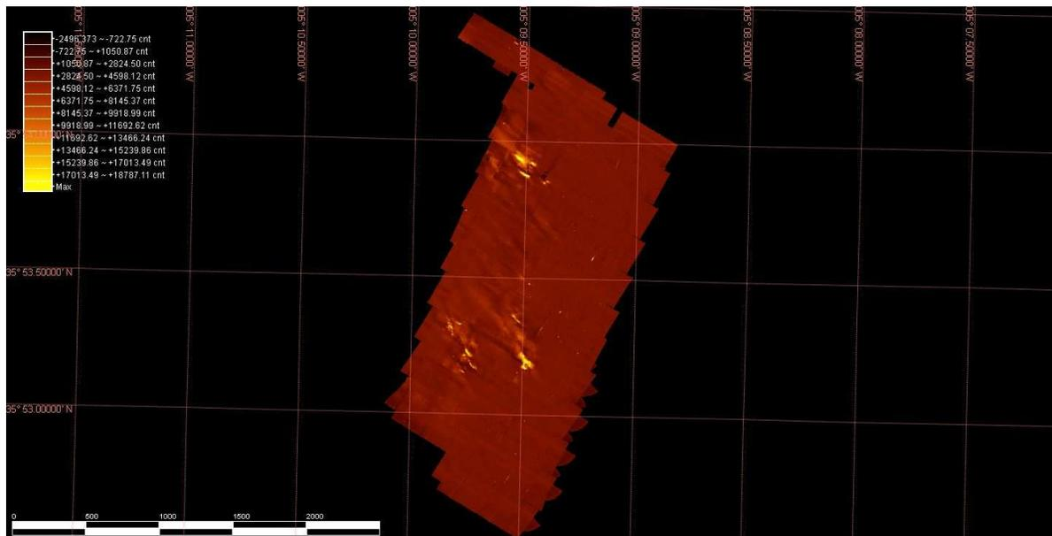
**Fig. 17** First processing of the data recorded on target area 2 (AUV dives 2.1 and 2.2). See figure 15 for location. The possible coral mounds are imaged in this mosaic. The reflectivity strongly suggests that the mounds have a rocky nature. A close-up on the mounds also reveals that the rocky mounds have an uneven, irregular texture.
