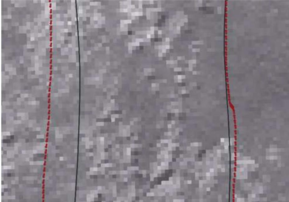
**Fig. 18** Example of the differences between the raw navigation of the AUV (dashed line in red), and the processed navigation (solid line in black). The maximum distance between the raw and the processed navigation in this capture is of 2.6 m.
