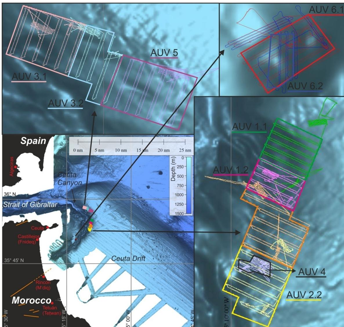
**Fig. 15** Location and tracks of the 10 AUV dives carried out for the GRACE Project during the course of the cruise. Of all the dives, 8 were carried out using the side scan sonar with long range, and 2 using the GAVIS Grasshopper camera (AUV 4 and AUV 6.2).
