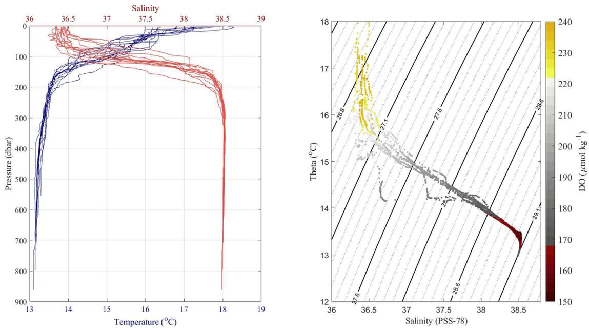
**Fig. 3** A) CTD temperature and salinity data of the 13 successful CTD profiles; B) T/S graphic of the CTD profiles, highlighting in yellow the Atlantic Waters and in red the Mediterranean Waters.
