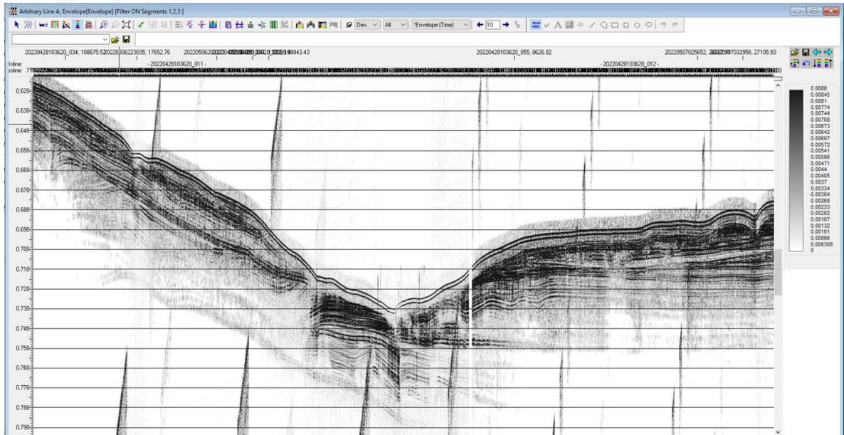
**Fig. 10** TOPAS acoustic profile roughly parallel to the canyon axis, showing one of the areas where the previous bathymetry hinted to sediment slides. The profile indicates that sediment slides have indeed occurred in the past.
