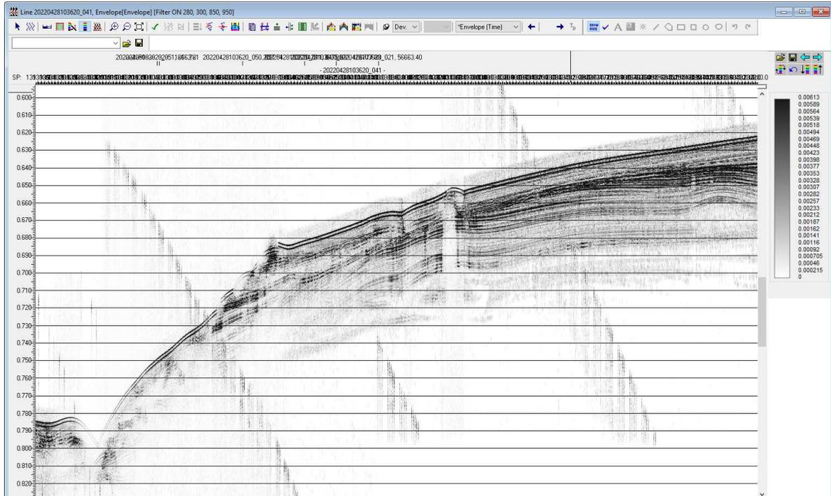
**Fig. 9** TOPAS acoustic profile roughly perpendicular to the canyon axis, showing one of the reliefs observed at the eastern axis of the canyon and providing further evidence of their nature as coral mounds.
