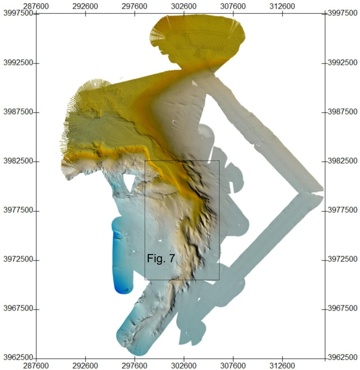
**Fig. 6** New preliminary multibeam map with 5 m resolution obtained after a first processing using CARIS HIPS & SIPS during the GRACE cruise.
