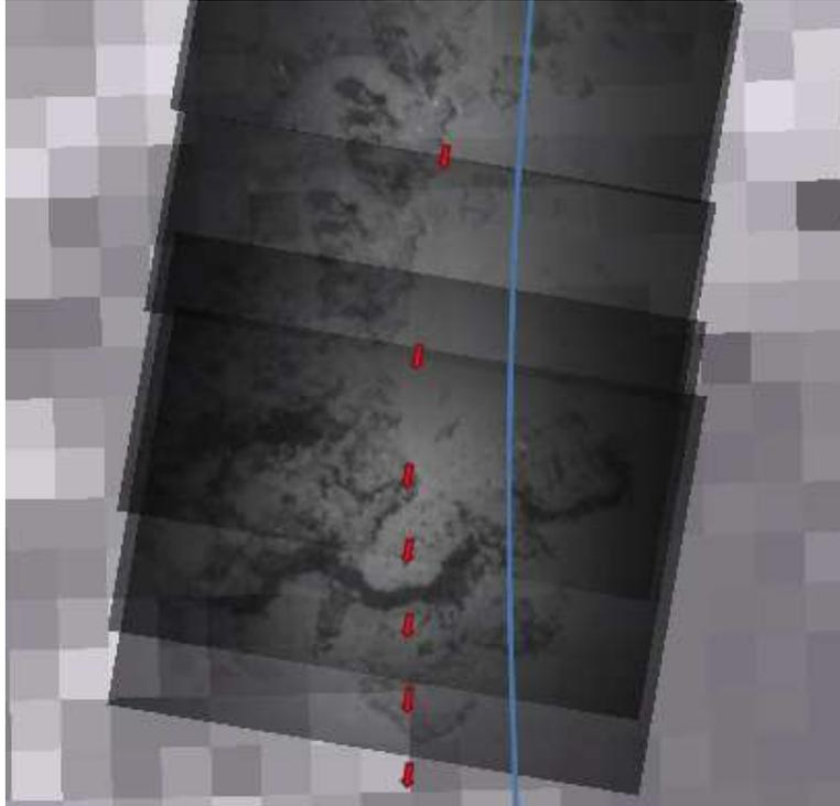
**Fig. 22** Example of a photo mosaic built using images recorded with the GAVIA grasshopper camera during AUV during Dive 02. The red arrows indicate the location of an image based on the uncorrected navigation files, with the tip of the arrow pointing the heading. The blue line shows the processed and corrected navigation line, where the images should be placed.
