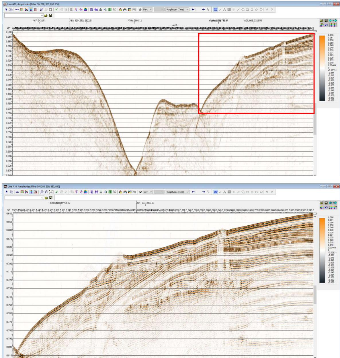
**Fig. 12** **A)** Cross-section of the Ceuta Canyon, showing atterraced plastered drift on the left (western side of the canyon) and possible coral mounds to the right (eastern side of the canyon). **B)** Detail of the possible coral mounds (both at the current seafloor and buried within the sediment); the Sparker line overlaps Fig. 9 (TOPAS), providing information of the same structure with different resolutions.
