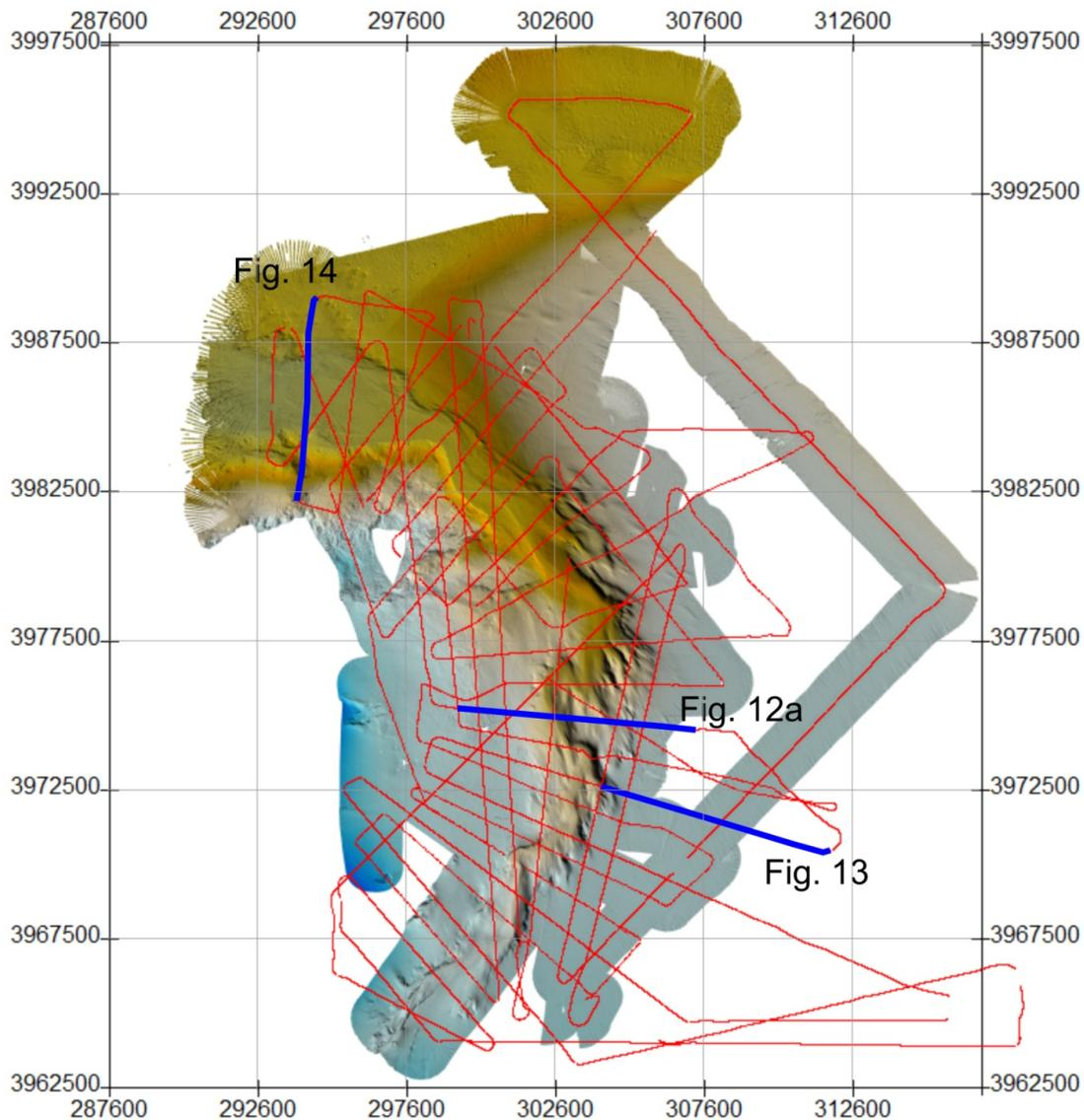
**Fig. 11** Overview of the Sparker single-channel seismic profiles recorded during the cruise.
