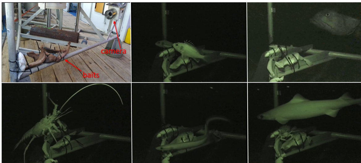
Figure 5.71: photo of the baited camera installed on the ALBEX 4 lander and selected frames of the recording periods.
