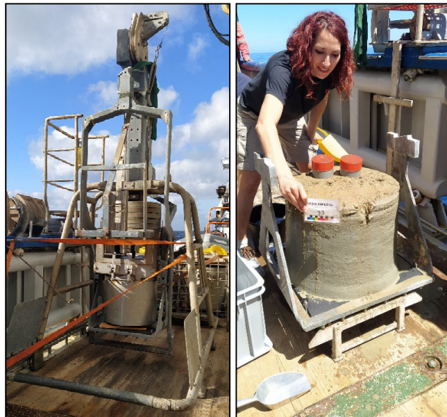
Fig. 5.77: photo of OASIS box corer and of Dr. Martina Pierdomenico working on the subsampling of OASIS box core 1 (station 73).
