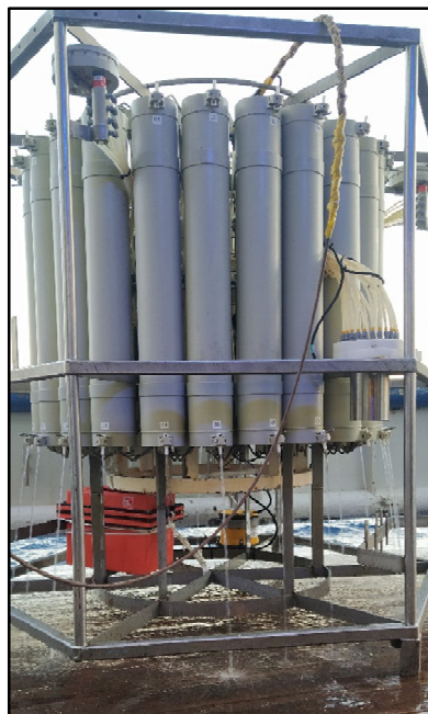
Figure 5.52: Photo of the CTD-rosette used during OASIS. L-ADCP is the yellow echosounder installed on the lower part of the frame. Red box is the battery pack supplying the L-ADCP.
