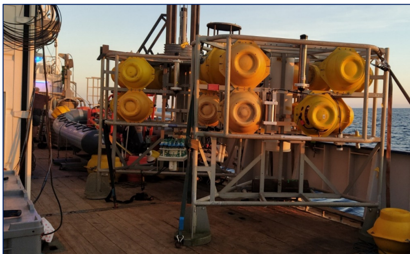
Figure 5.67: The two ALBEX benthic landers used in OASIS soon before their deployments.
