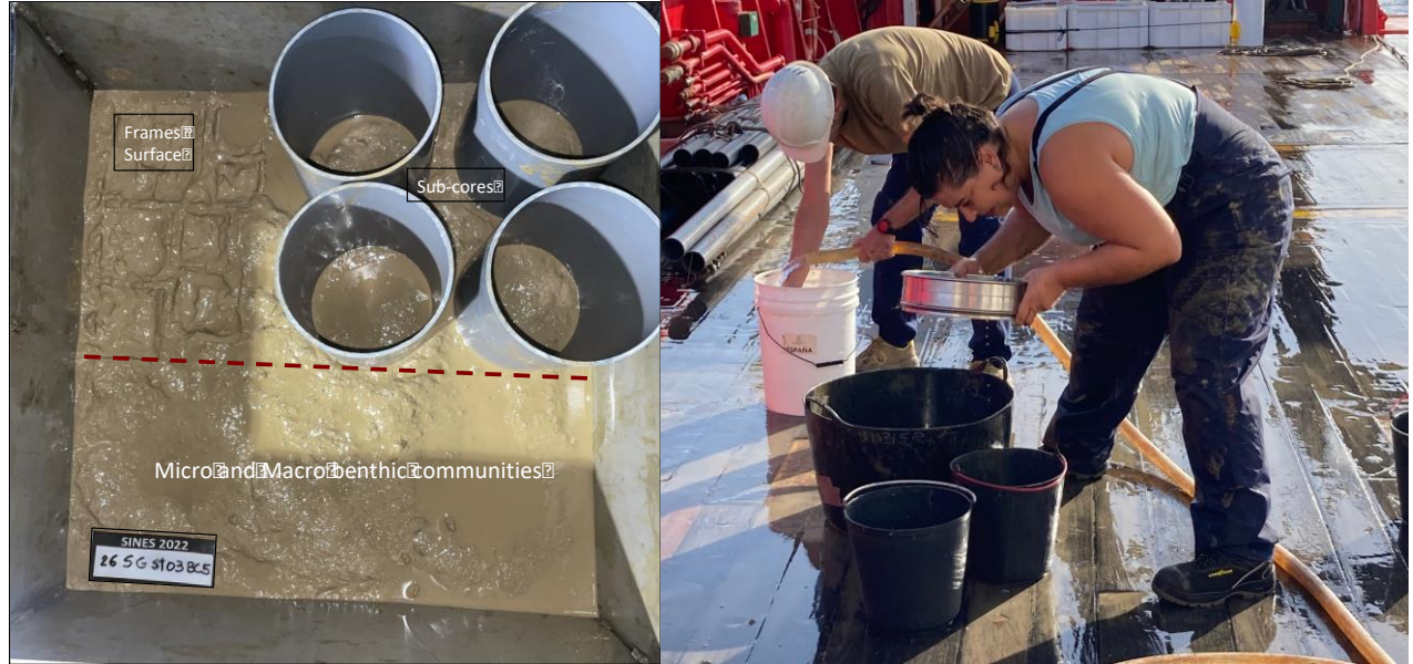
Figure 13 – (left) Example of a box-core sampling strategy; (right) Washing sediment through a 250 µm mesh for micro and macro benthic communities' separation.
