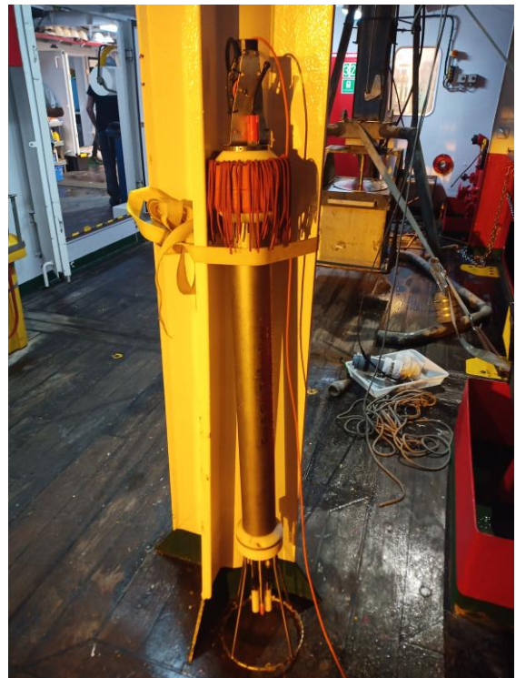
Figure 15 - The microstructure vertical profiler (MSS-90) on deck.
