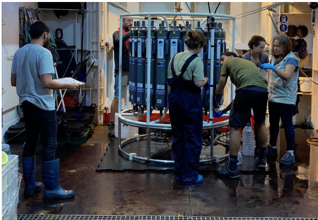
Figure 8 – Seawater sampling from the CTD-Rosette system with 24 Niskin bottles of 12 L each. Sea water collected at different levels is retired from the bottles by the different research groups according to the plan presented in Table 1.
