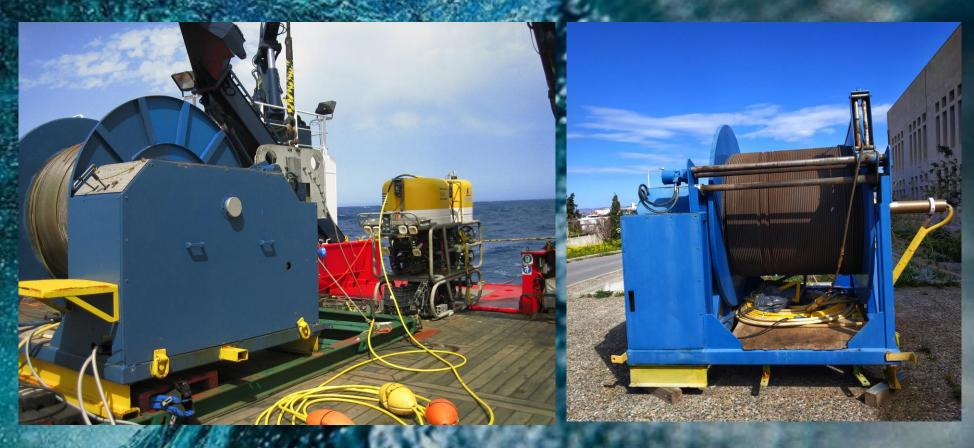
The winch is responsible for diving the rigid cable and submersible robotic vehicle in the water.
