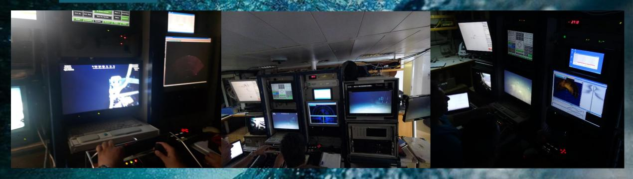
The system control consists from consoles needed for controlling the ROV, recording different types of scientific data and carrying out sampling and measurements.
