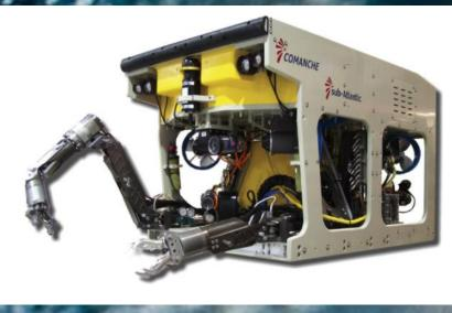
**Shallow MSROV**: Low-power vehicles with copper (or fiber) telemetry and ,1000 m depth capability
