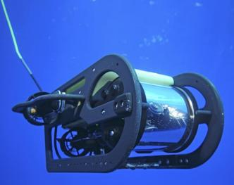
Depth Rating 200 m 530 mm Length 245 mm Width 254 mm Height Weight in Air 11 kg
