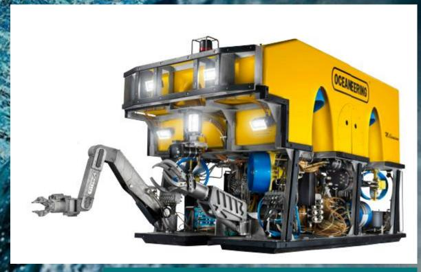
**Heavy work class:** These vehicles are very large and heavy work vehicles of 200 hp or greater for heavy construction work
