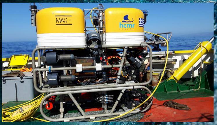
Depth rating 2000 m 2200 mm Length Height 2000 mm 900 mm Width Weight in air 1100 kg Payload 68 kg Underwater speed: 2.5 knots (fwd/rev),1.5 knots (vert/lat)
